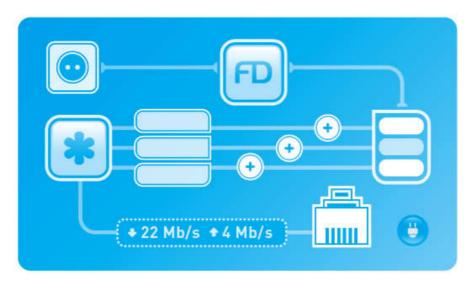
The PureFluid service is presented to your network via a single Ethernet connection (using Cisco 2800 series router) with a single static IP block applied to the overall service. This allows for seamless failover. If one of the composite circuits develops a fault your IP routing remains unaffected as PureFluid continues using the working circuits. This failover happens so quick that VoIP, VPN and even video traffic is unaffected.
